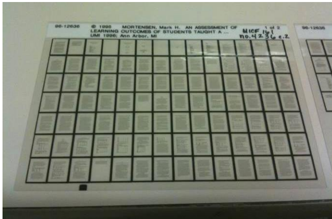
Microfiche, a less common counterpart to microfilm, is printed on flat sheets of film.
